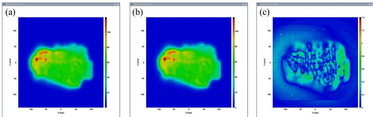
Fig. 2: Dose verification results for a large IMPT field (sacral chordoma case). (a) Calculated dose, (b) dose measured with CCD beam imaging system and (c)  $\gamma$ -Evaluation with  $\Delta D=3\%$  and  $\Delta d=3\text{mm}$  acceptance criteria for maximum dose and distance deviations.
