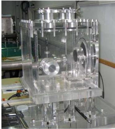
Figure 7 PMMA phantom of the BIPM calorimeter. The small graphite cylinder on the right is the jacket and the larger disc is the entrance window. Image courtesy BIPM [10].
