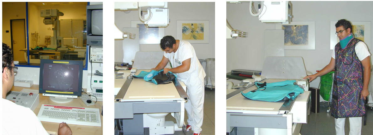
Figure 3: Testing X-Ray protection clothing using a fluoroscopy unit
