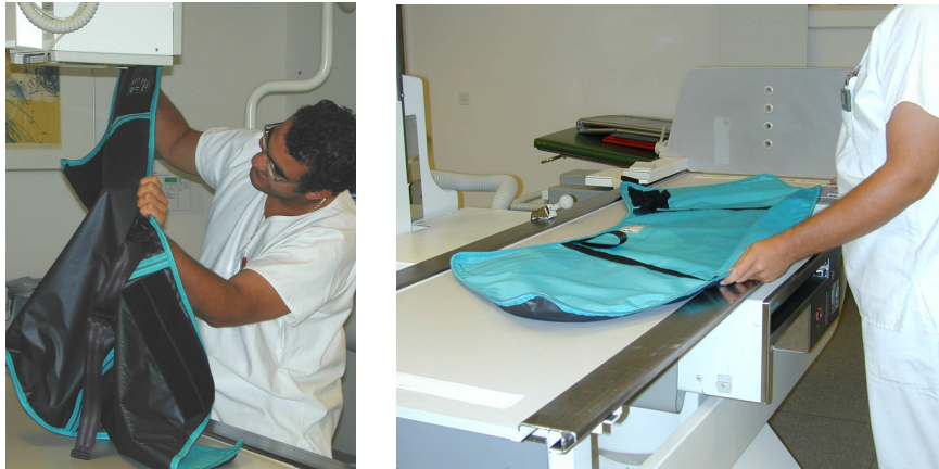
Figure 2: Testing X-Ray protection clothing by visual inspection and palpation
